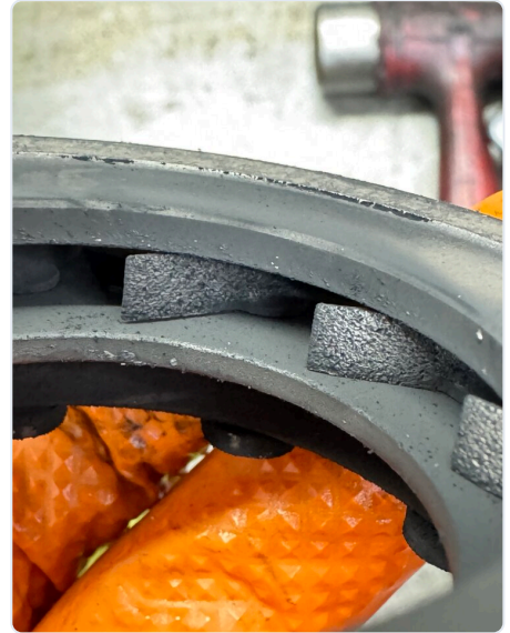
Fig. 3 - Variable geometry components: heat exposure and discolouration.
