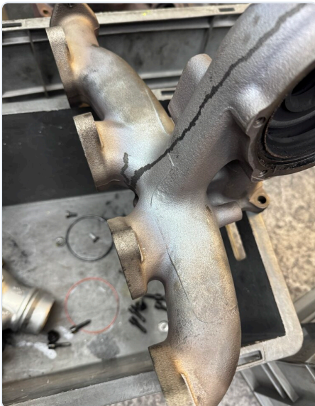
Fig. 4 - Turbine / exhaust housing: evidence of excessive thermal loading.
