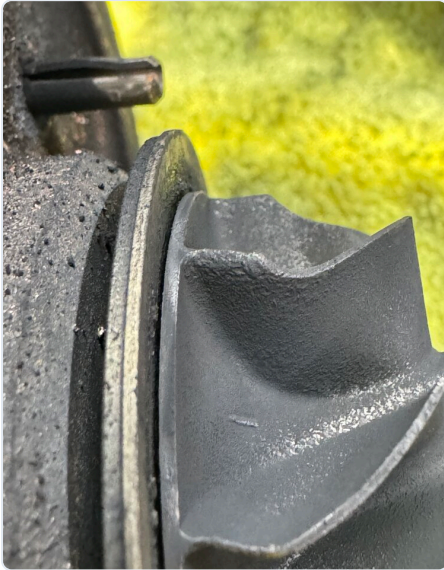
Fig. 1 - Turbine wheel / shaft area: visible heat-related surface damage.
