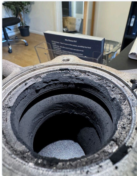
Fig. 5 - Heavy carbon contamination inside the turbine / exhaust housing.
