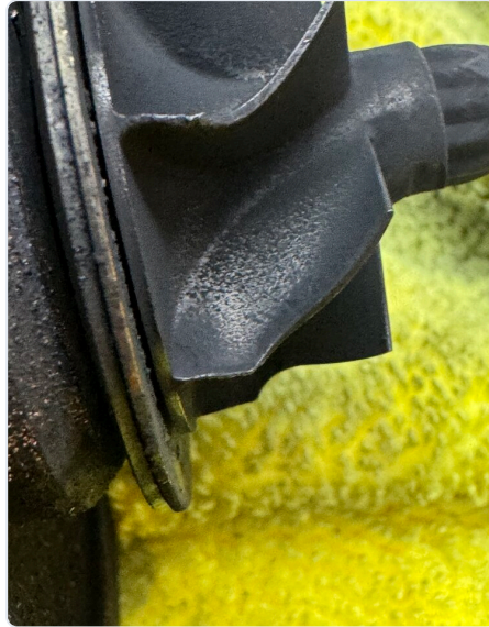
Fig. 2 - Turbine wheel detail: abnormal surface condition and thermal exposure.
